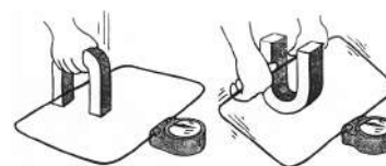
Fig. 11.16: Voltage is induced in the wire loop whether the magnetic field moves past the wire or the wire moves through the magnetic field.
