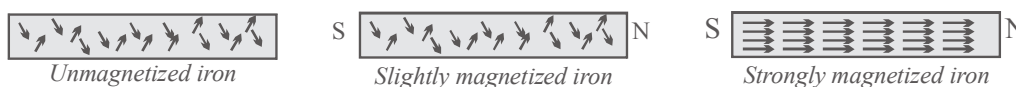
Fig. 11.5 : Pieces of iron in successive stages of magnetism. The arrows represent domains; the head is a north pole and the tail is a south pole. Poles of neighboring domains neutralize each others effects except at the ends.
