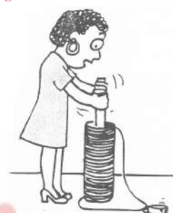
Fig. 11.18 : It is more difficult to push the magnet into a coil with many loops.
