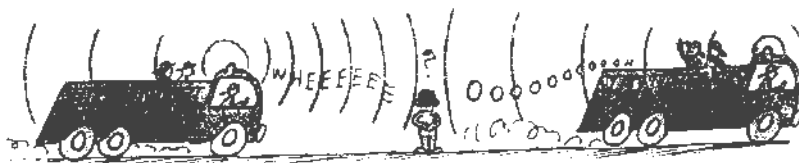
Fig. 3.6 : The pitch of sound increases when the source moves towards you, and it decreases when the source moves away
