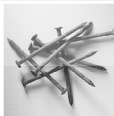
Rusting of iron nails
